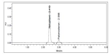
Fig 2: Typical chromatogram of Netupitant and Palanosetron
