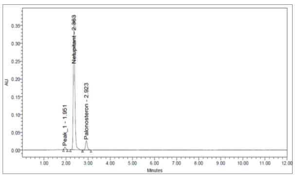
Fig 5: Peroxide degradation chromatogram of Netupitant and Palanosetron
