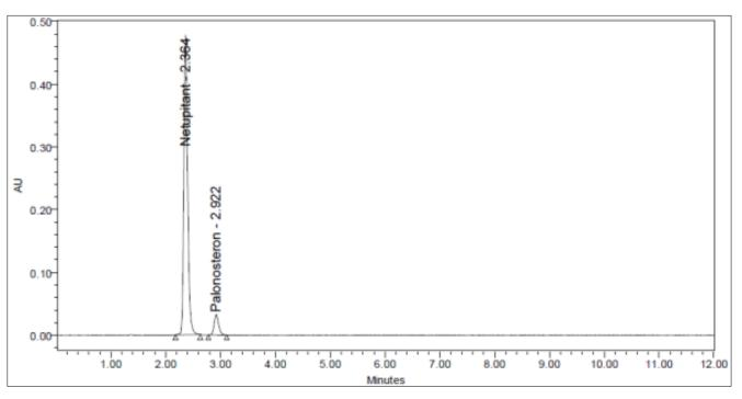
Fig 6: Water degradation chromatogram of Netupitant and Palanosetron
