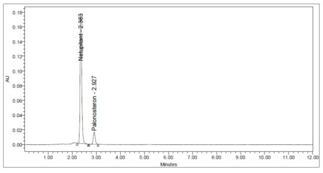
Fig 4: Base degradation chromatogram of Netupitant and Palanosetron
