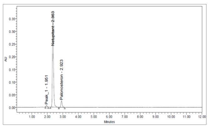
Fig 7: Thermal degradation chromatogram of Netupitant and Palanosetron
