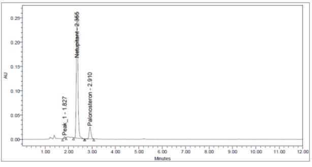
Fig 3: Acid degradation chromatogram of Netupitant and Palanosetron
